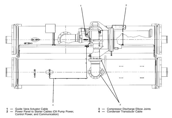
Fig. 7 — 19XR Chiller Top View
